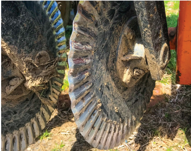
Figure 2: Fluted coulter disc found on a no-till drill to help cut through sod and hard soil ahead of the openers.
