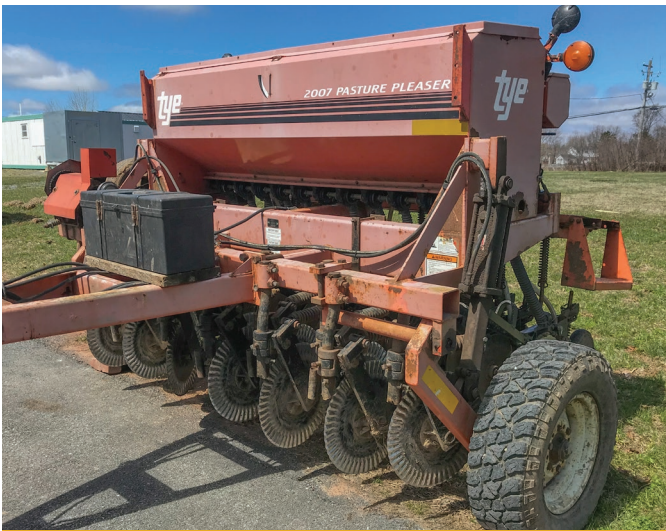
Figure 1: Tye no-till drill suitable for no-till interseeding pastures and hayfields
