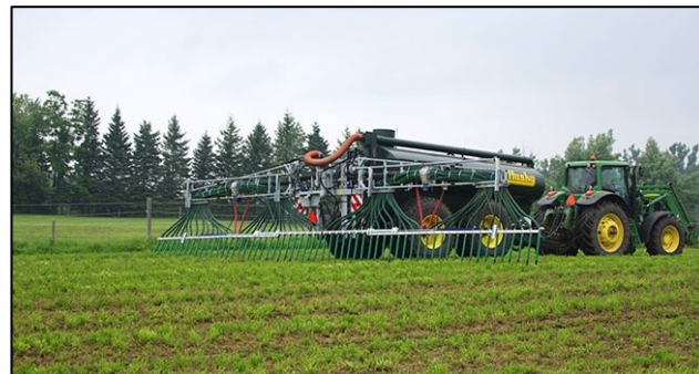
Figure 1: Dribble bar applicator (Photo: Manure Manager )
